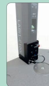
LABI-SAC Subwoofer to column adapter
