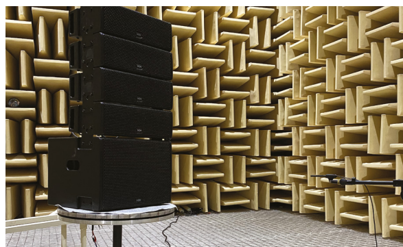
TNA-2051 & TNA-1200S SOUND TEST IN ANECHOIC CHAMBER
